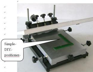
2.) Put the simple DIY positioner on the printing table and also put the PCB accordingly. Adjust the five-star handle on the operation platform to make the holes on PCB match the holes on the steel stencil.
