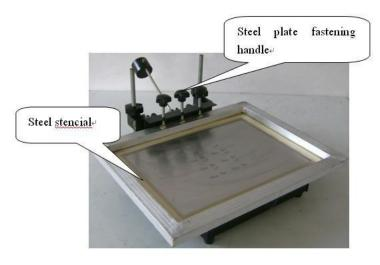
1.) Put steel stencil in the wire clip, and tighten the steel stencil by its handwheel.
